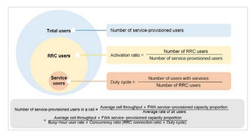
Figure 3: Model of the number of users for which wireless FWA service can be provisioned
