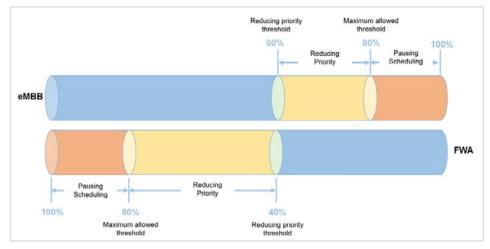
Figure 9: QoS PRB control solution for multi-service networks
